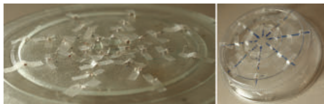
Figure 5. A turntable with 32 neon lights (left) and a plate cover with 32 neon lights (right).
