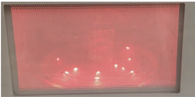
Figure 6. The turntable inside a running oven. The brightness of a neon light is proportional to the EM-field strength at the placed location.
