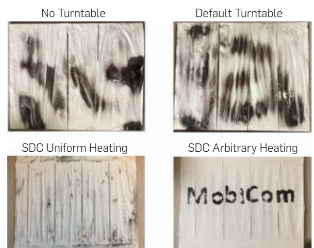
Figure 1. Results of microwaving wet thermal paper (black spots indicate high heat). (Top) A traditional microwave without/with a turntable. A turntable can mitigate uneven heating, but cold/hot spots remain. (Bottom) SDC, for uniform heating (fewer black spots show heat is spread uniformly) or heating to write "MobiCom." We use patterned susceptors and let SDC ensure the text area has been heated in hot spots.
