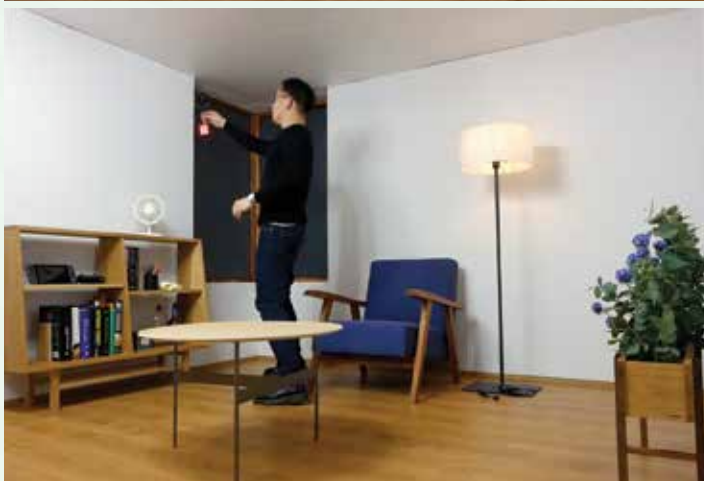
Multi-mode Quasistatic Cavity Resonator uses a room's walls, floor, and ceiling as low-loss transmission resonators to send tens of watts of power anywhere in a three-meter square room.
