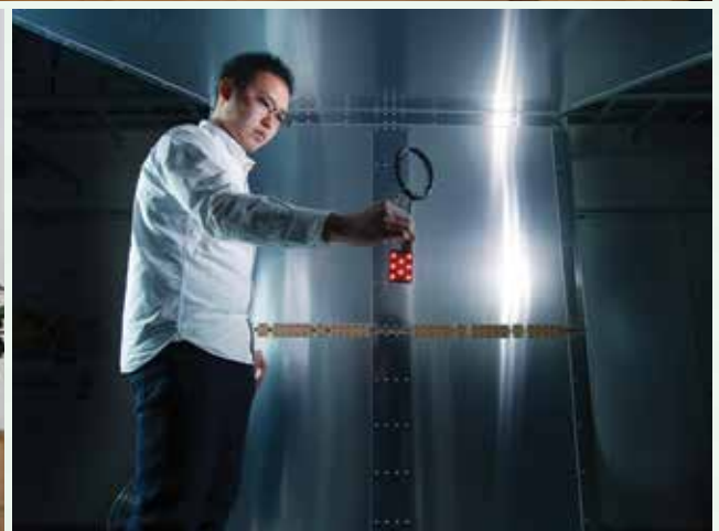
Multi-mode Quasistatic Cavity Resonator uses a room's walls, floor, and ceiling as low-loss transmission resonators to send tens of watts of power anywhere in a three-meter square room.
